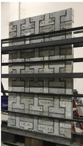
Figure 2. The 1-D TeSA wall specimen (image by author) [9].
