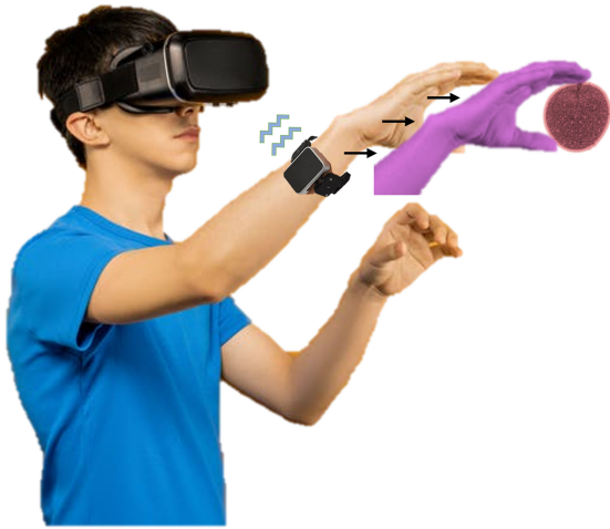
Fig. 1. The interaction-expectation model predicts contact with a virtual object before it occurs. As a demonstrative example, the user begins reaching for the virtual apple. We predict the interaction before it occurs. This information can be communicated to a haptic device (picture from [10]), so it can provide haptic feedback at the correct time, unhindered by sense-to-actuation latency.
