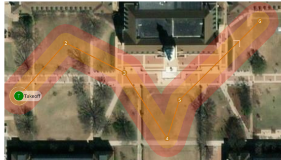
Figure 9. Altered risk buffer with different colors and larger buffer radii.
