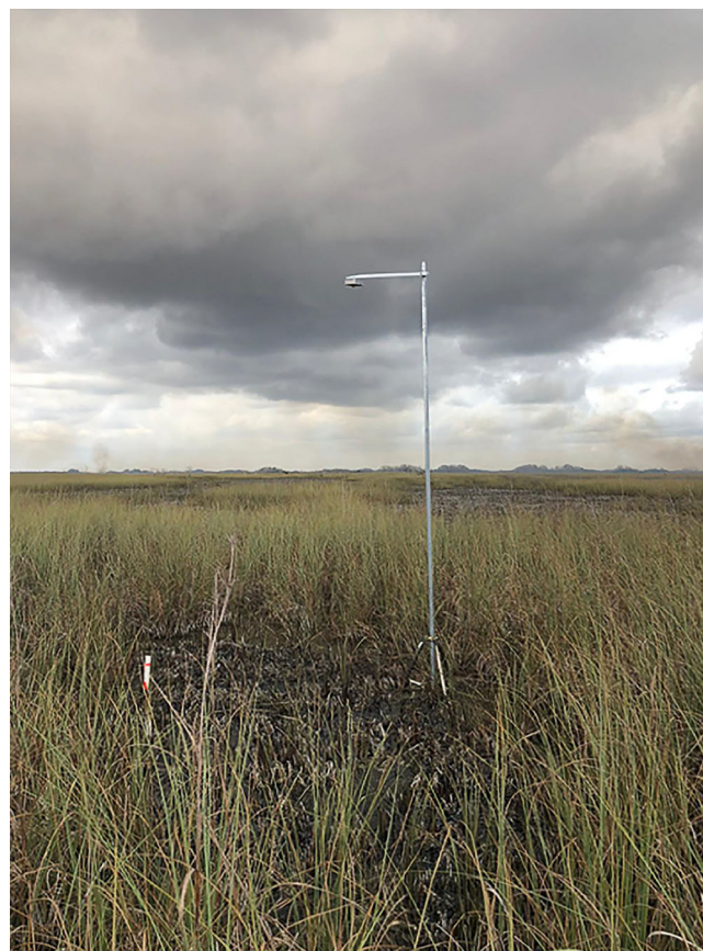
FIGURE 2 One of the infrared radiometers, set up on top of a tripod, at one of the experimental plots of the lower-P site, pictured after the prescribed fire carried out on 18 February 2020 in the eastern marl wetlands of the Everglades (Florida, USA). Infrared radiometers were used to measure fire radiative power and energy, which we used to express fire intensity. In this picture, the patchiness, which characterized the entire fire, is clearly visible. Photo credit: Andrea Nocentini.
