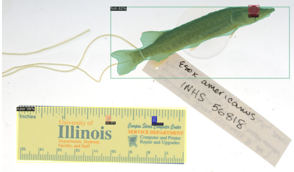
Fig. 2. Initial object detection on a specimen image using Detectron2 [34].
