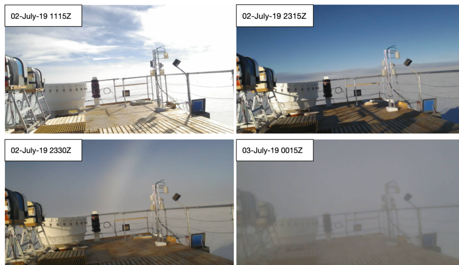
Figure 12. Photographs from a webcam oriented towards the eastern horizon on 2 and 3 July 2019. The aerosol inlet is visibly mounted on the mast in the SE corner.
