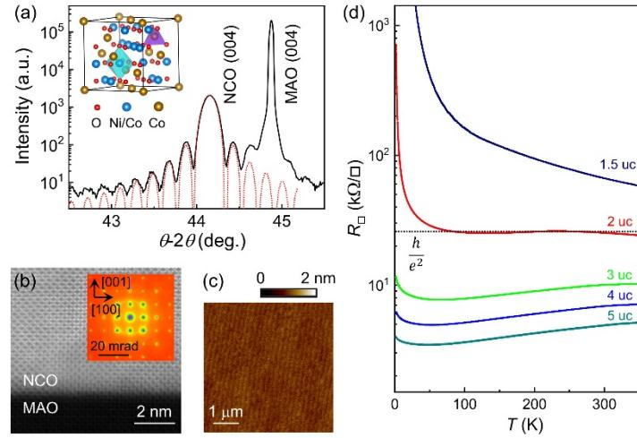
**FIG. 1.** (a) XRD  $\theta$ - $2\theta$  scan of a 60 uc NCO film on MAO with a fit to Laue oscillations near the (004) peak (dotted line). Inset: Schematic of NCO crystal structure. (b) HAADF-STEM and (inset) SAED images taken on a 17 uc NCO. (c) AFM topography image of a 5 uc NCO showing atomically flat terraces. (d)  $R_{\square}(T)$  for 1.5-5 uc films. The dotted line illustrates the two-dimensional quantum resistance  $\frac{h}{e^2}$ .
