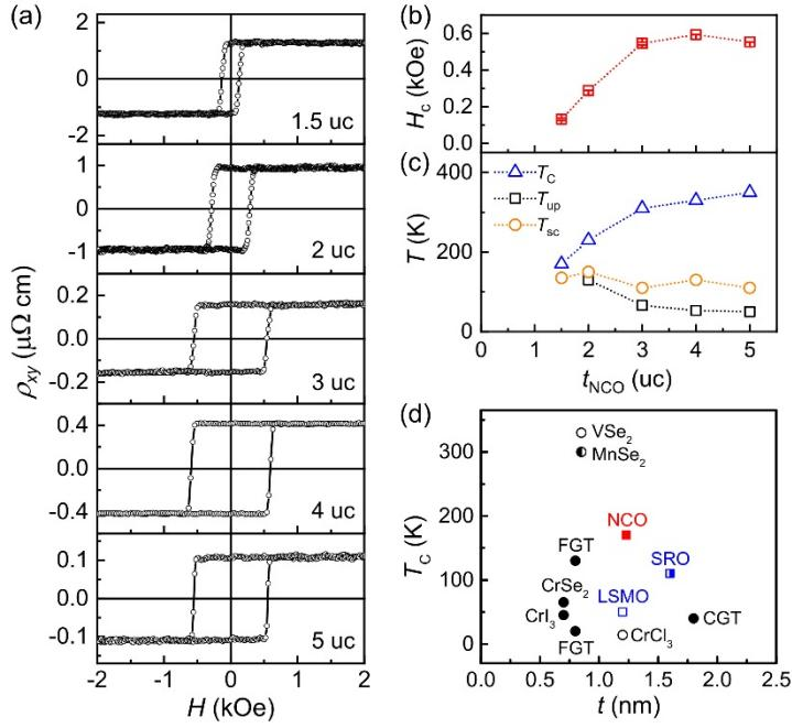
**FIG. 2.** (a)  $\rho_{xy}$  vs  $H$  hysteresis at 100 K for 1.5-5 uc NCO. (b-c)  $t_{NCO}$ -dependence of (b)  $H_c$  at 100 K, and (c)  $T_c$ ,  $T_{up}$ , and  $T_{sc}$ . (d)  $T_c$  vs. thickness for epitaxial complex oxide films (squares)<sup>24,25</sup> and 2D vdW magnets (circles).<sup>26-33</sup> Solid symbols: PMA. Open symbols: in-plane MA.
