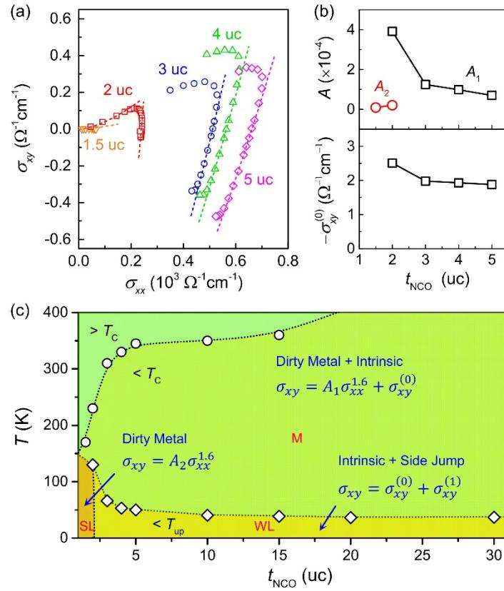
**FIG 4.** (a)  $\sigma_{xy}$  vs.  $\sigma_{xx}$  for 1.5-5 uc NCO films with fits to Eqs. (2)-(3) (dash lines). (b)  $t_{\text{NCO}}$ -dependence of  $A_1$ ,  $A_2$  and  $\sigma_{xy}^{(0)}$ . (c) Temperature-thickness diagram of the AHE scaling behavior. M: metallic. WL: weakly localized. SL: strongly localized. The data for 10-30 uc films are taken from Ref. [3].
