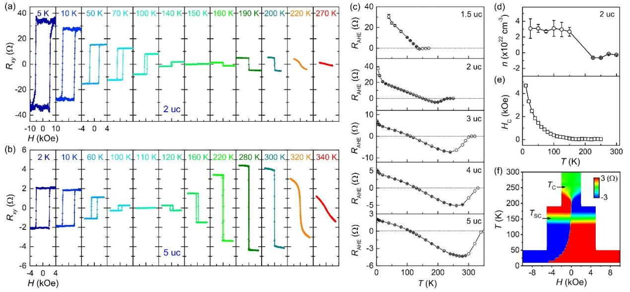
**FIG. 3.** (a) AHE of 2 uc NCO at various temperatures. Field range:  $\pm 10$  kOe for 5-10 K and  $\pm 4$  kOe for higher temperatures. (b) AHE of 5 uc NCO at various temperatures. (c)  $R_{AHE}$  vs.  $T$  for 1.5-5 uc NCO. (d)  $n$  vs.  $T$  and (e)  $H_c$  vs.  $T$  for 2 uc NCO. (f)  $R_{xy}$  vs.  $T$  and  $H$  (sweeping down) for 2 uc NCO.
