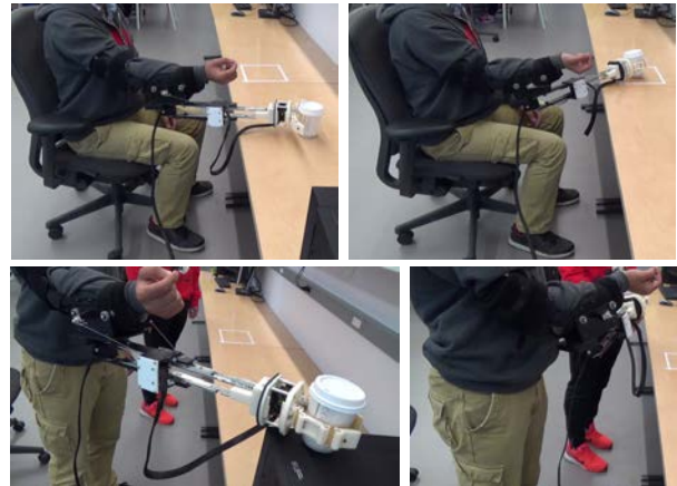
Fig. 8. Tasks performed by users: moving a cup on a table while seated, and handing over a cup to the interviewer while standing.
