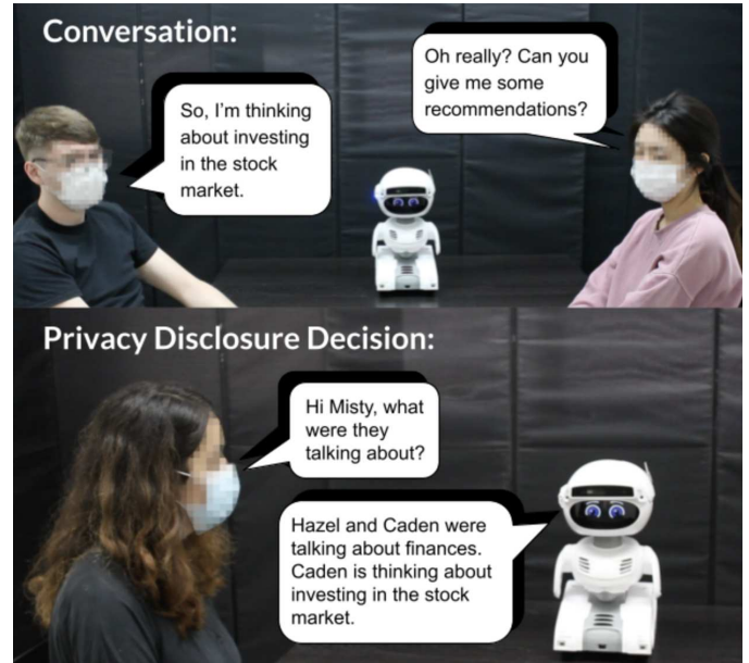
Fig. 1. In this paper, we design a privacy controller for social robots. Here, the robot processes a set of metadata extracted from a conversation and decides the privacy state of this conversation. Using this privacy state, the robot can determine whether information can be appropriately shared with other users. We evaluated the effectiveness of the design with two user studies.
