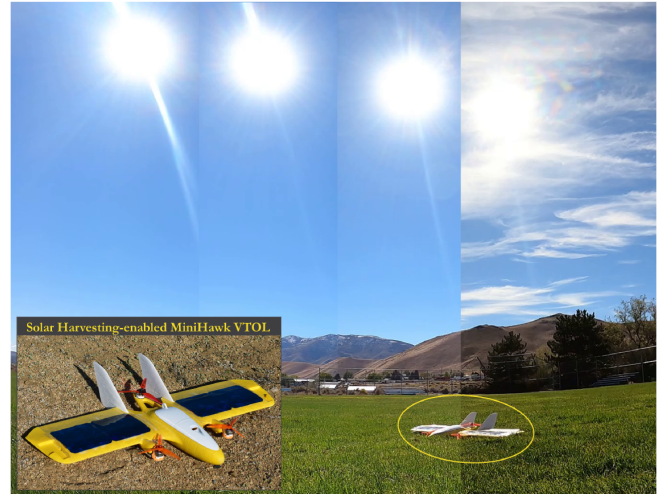
Fig. 1. The MiniHawk-VTOL, a Tri-TiltRotor hybrid aircraft equipped with onboard solar energy harvesting for migratory (recurrent-mission) behavior demonstration.
