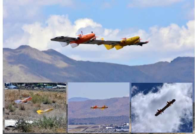
Fig. 1. The Aspect Ratio-Modular Vertical Take-Off and Landing (ARM-VTOL) reconfigurable aerial robot, consisting of a pair of wingtip-to-wingtip connected Tri-TiltRotor hybrid aircraft. Corresponding video available at: https://www.youtube.com/watch?v=pVbJdrOTGY
