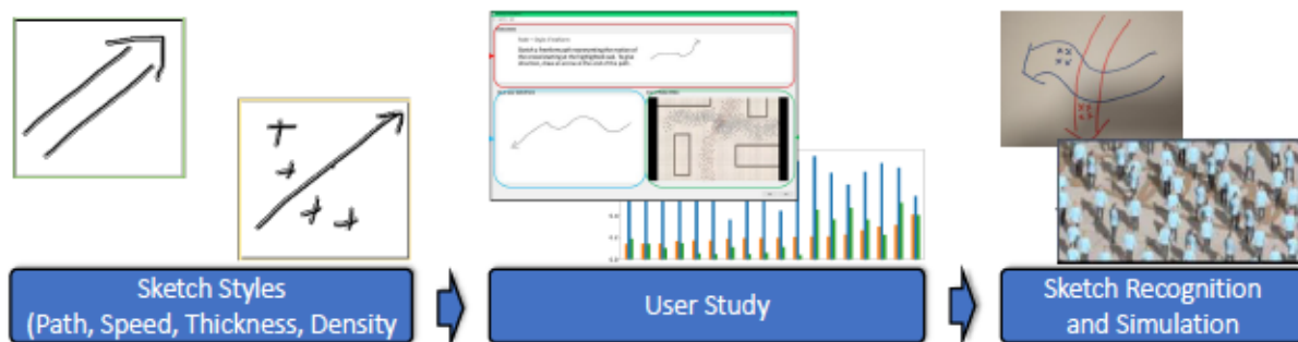
Figure 1: Sketching Vocabulary for Crowd Motion: This paper proposes various intuitive sketch styles for specifying crowd motion parameters defining motion path, walking speed, path thickness, and crowd density ("Sketch Styles"). A prototype system pipeline converts sketches into parameters for a crowd simulation and animation ("Sketch Recognition to Crowd Simulation") and it reports the best styles, and relevant observations, as per a user study ("User Study and Results").
