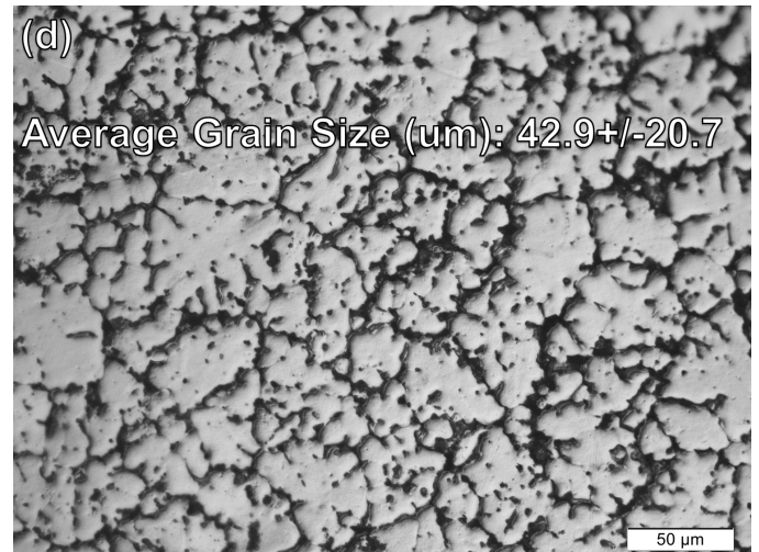
Figure 6: Etched micrographs within regions of interest from etched macrograph (Figure #): location 1 (a) location 2 (b) location 3 (c) location 4 (d) with average grain size. Sample [232]
