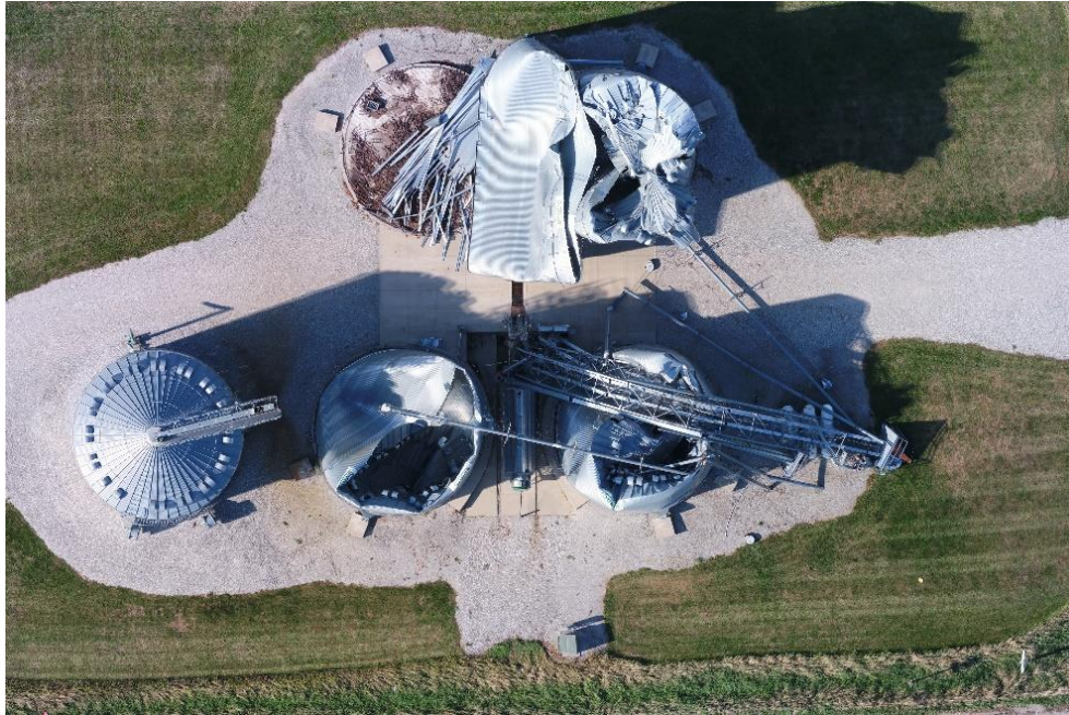
Figure 5. Orthomosaic of case study site following August 2020 derecho.
