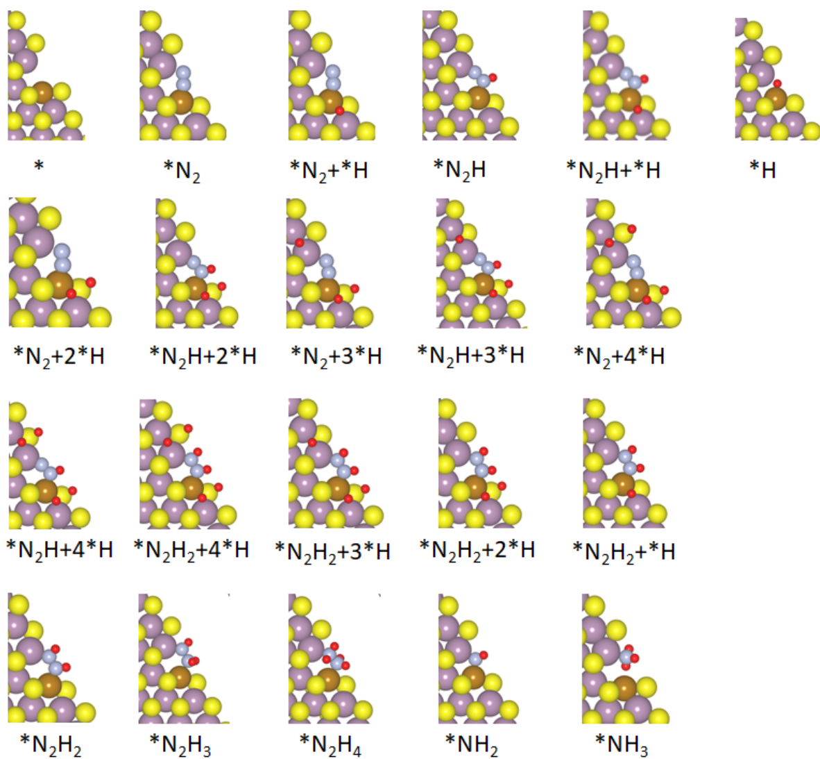
Figure S8. Top view of the V_s@1Fe-S50 site with various NRR intermediates corresponding to the reaction network in Figure S5. Gold, red, violet-grey, yellow, and silver spheres represent the Fe, H, Mo, S, and N atoms, respectively.
