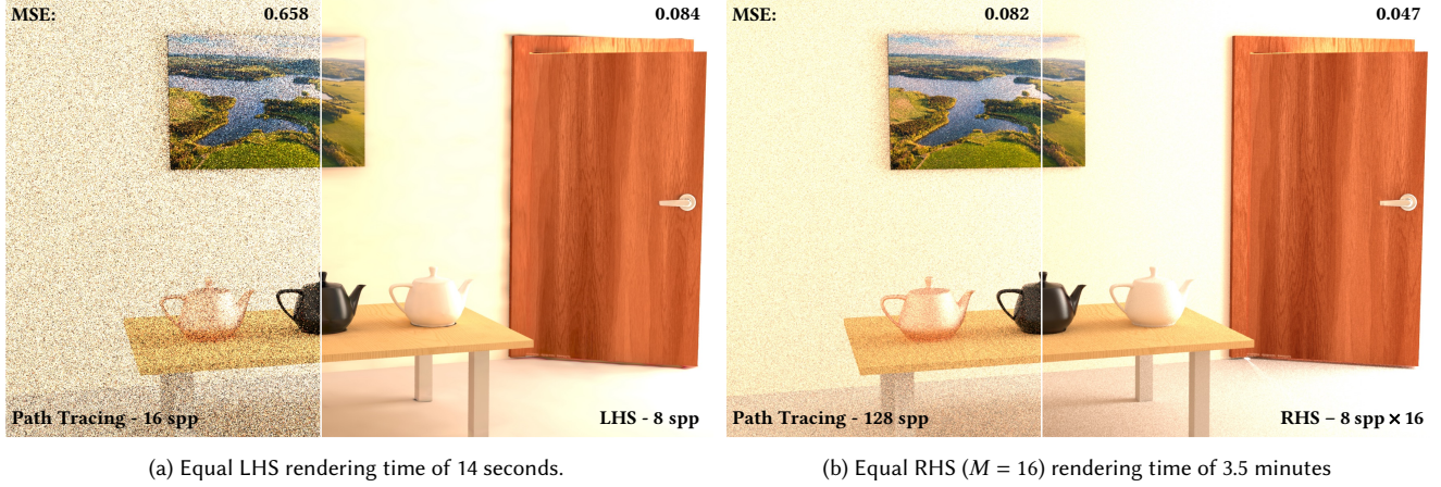
Fig. 8. Equal rendering time comparison between our pre-trained model and path-tracing. The training time for the model took about 3 hours (Table 1). As an implementation detail, note that the rendering time depends on parameters such as the GPU thread block size. To use larger spp, we must accommodate GPU memory availability by dividing the computation into smaller blocks. Thus, 128 spp path-tracing is not exactly 8 times as costly as 16 spp.
