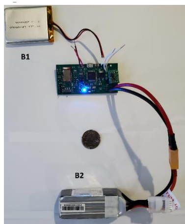
Figure 8. Photo of the final PCB with two batteries, B1 and B2. The 3.7 V battery (B1) powers the microcontroller and Bluetooth module. The 14.8 V battery (B2) powers the solenoid.
