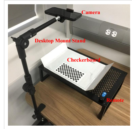
Fig. 3. Experiment setup for \overline{\text{OIS}} image collection.
