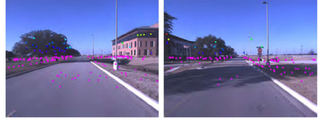
Fig. 6. A sample of camera image data captured simultaneously with the radar data by our autonomous vehicle platform during the physical experiments. The colored points are the radar target detections projected into the image coordinates. Note that the target elevations are the absolute elevations as estimated by (13). The point color coding indicates the target's height in meters relative to the horizontal plane. Projected images are generated by RViz.
