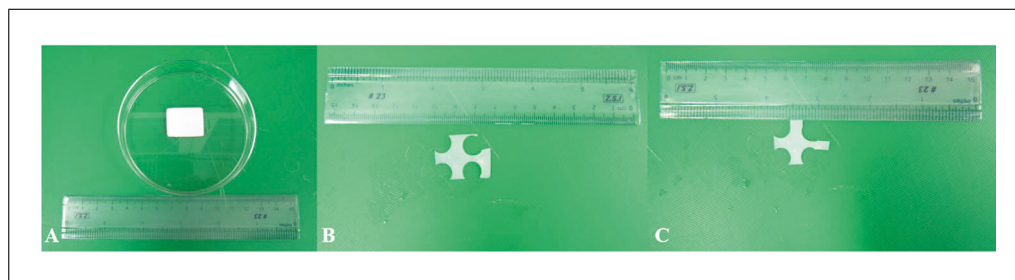
Figure 8 (A) Place the TissueMend in a petri dish, cover with room-temperature PBS, and allow 10 min for the sample to become fully hydrated. (B) Using a biopsy punch, remove the corners of the rectangular analog to create a roughly cruciform-shaped sample. (C) Use a razor blade to trim away excess material, yielding the desired cruciform shape.
