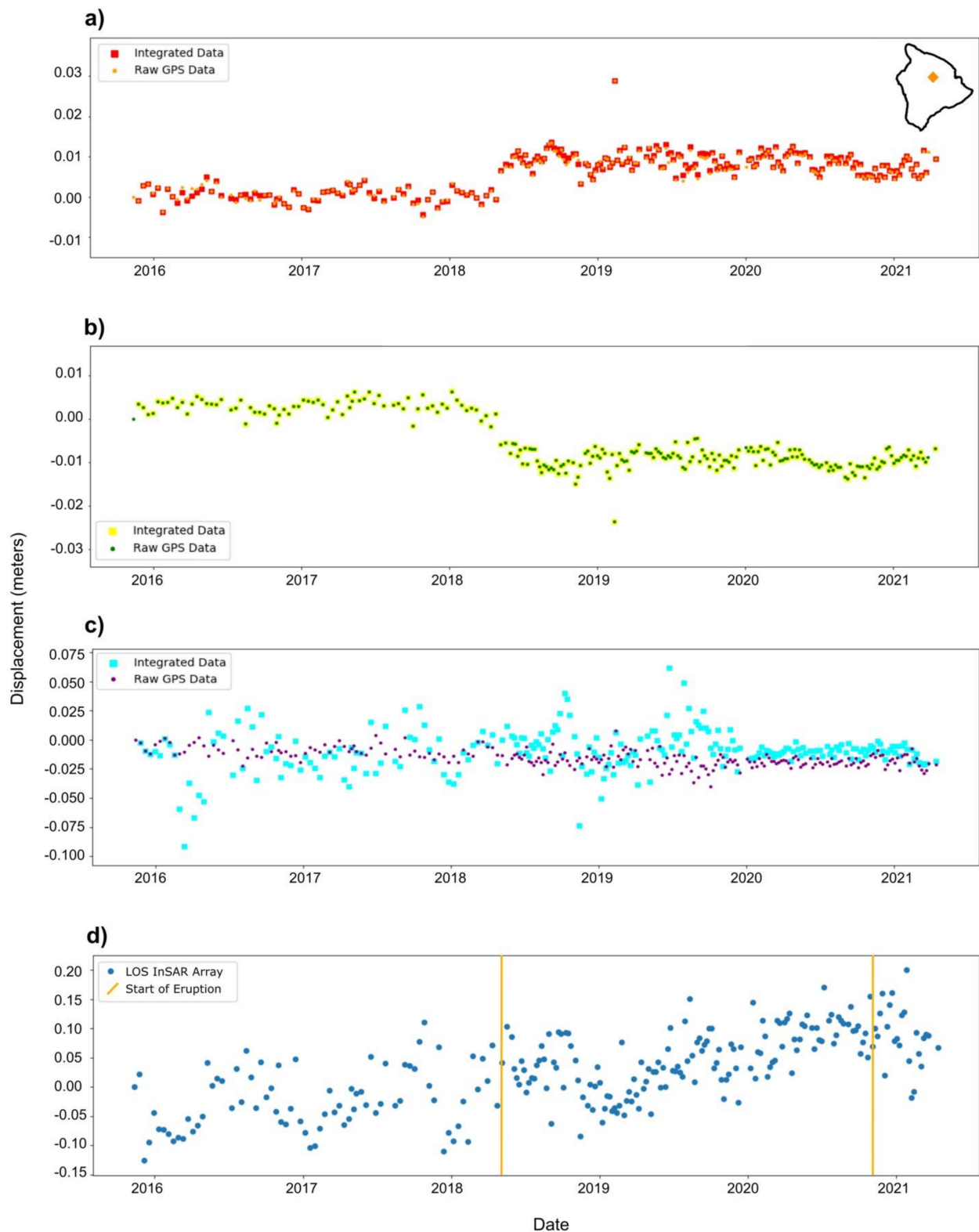
Figure 10. Integrated results compared to original, raw GNSS time series in the (a) east-, (b) north-, and (c) up-components of motion at MKEA GNSS station ( 19.801^{\circ}\text{N} , -155.456^{\circ}\text{W} ). Motion in the east-west and north-south directions are slightly more constrained, while motion in the up-down direction is significantly transformed after combining the DInSAR and GNSS datasets together. (d) DInSAR LOS time series at the same pixel, MKEA station. Yellow lines are as in Figure 8, above. The inset in subfigure a shows location of MKEA station in Hawaii.
