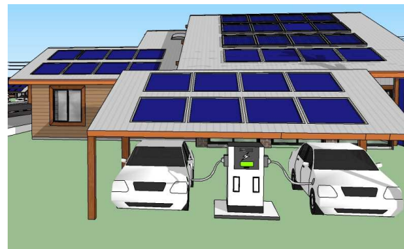
Fig. 1. DC fast charging station using PV to Vehicles
