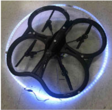
Fig. 3. Picture of UAV with blinking LED marker ring.
