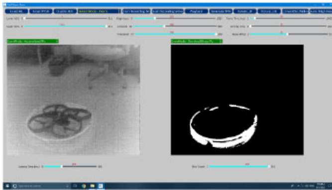
Fig. 2. Graphical User Interface of the Celex Dynamic Vision Sensor showing both normal image and temporal difference image of the blinking LED Marker.
