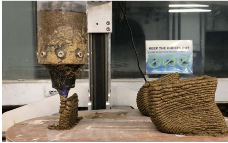
Figure 7: Printing in progress of angled tests and single layer buildability test.
