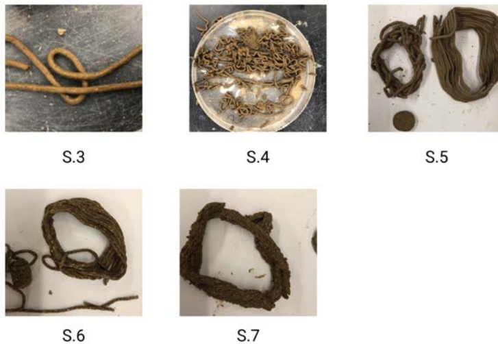
Figure 6: Extrusion tests of subsoil mixtures
