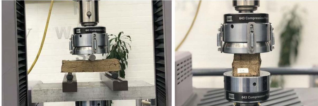
Figure 8: compressive and flexural strength tests using MTS Criterion C43 Electromechanical Testing Machine.
