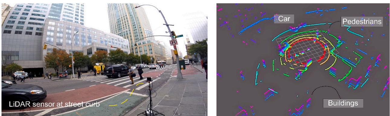
Fig. 3. Site observation in Brooklyn, NY. (Left) video scene; (Right) LiDAR data from the scene.
