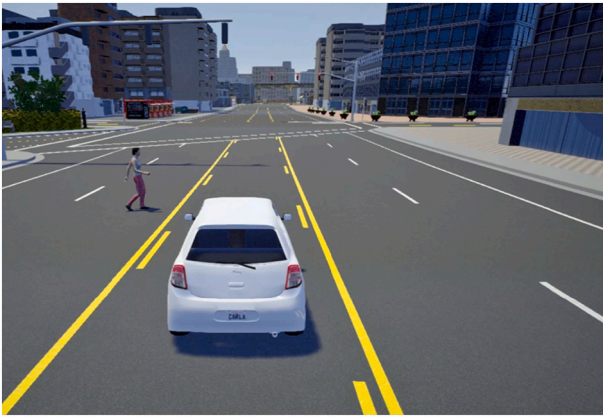
Fig. 25. Our implementation of the CARLA driver behavior model with geographic automata pedestrian simulation in the system. The pedestrian is jaywalking and the vehicle has detected this and come to an abrupt stop outside of its usual traffic signal event.
