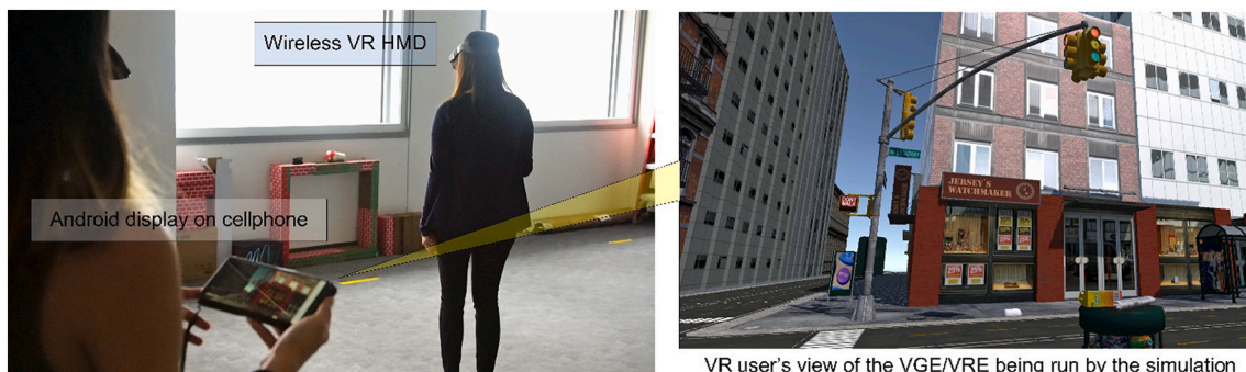
Fig. 26. Wireless implementation of the system on the Oculus HMD and a remote Android viewscreen.
