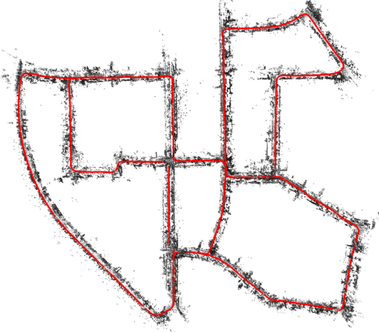
Fig. 1. The estimated trajectory and reconstructed environment by the proposed method on KITTI sequence 00.
