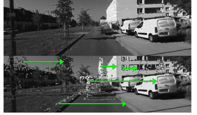
Fig. 3. An example of scale optimization on sequence 06 of the KITTI dataset. The top image is the projection with the optimal scale, where the projection well overlaps with the image; the bottom image is the projection with an incorrect scale ( 0.1 \times optimal scale), the green arrows indicate the locations of the correct projections.
