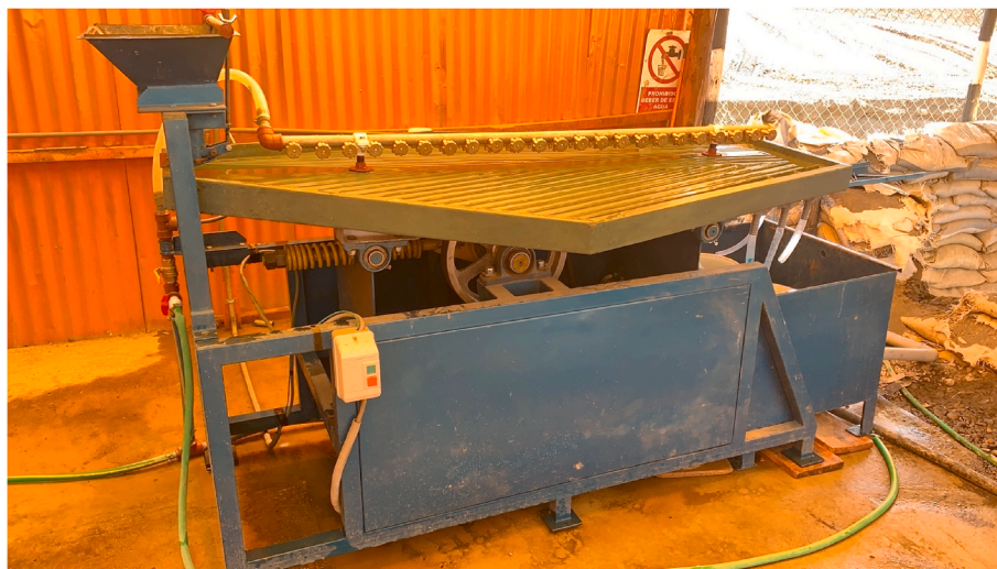
Fig. 2. In September 2019, one Fairmined cooperative implemented a shaking table to further concentrate their pre-concentrates obtained from the sluices and remove the use of mercury. After a small high-grade gold concentrate is obtained, the cooperative uses borax to recover gold. (For interpretation of the references to colour in this figure legend, the reader is referred to the Web version of this article.)
