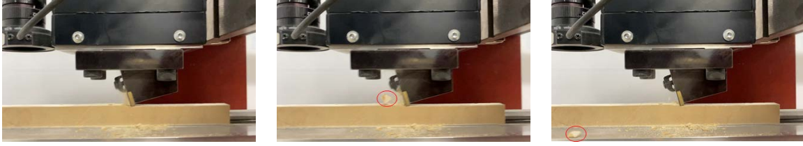
Figure 15: Identification of the formation for flake-like fragments at a depth of cut 1.0 mm via reviewing the recorded videos. The flake-like chip is marked by the red circle.
