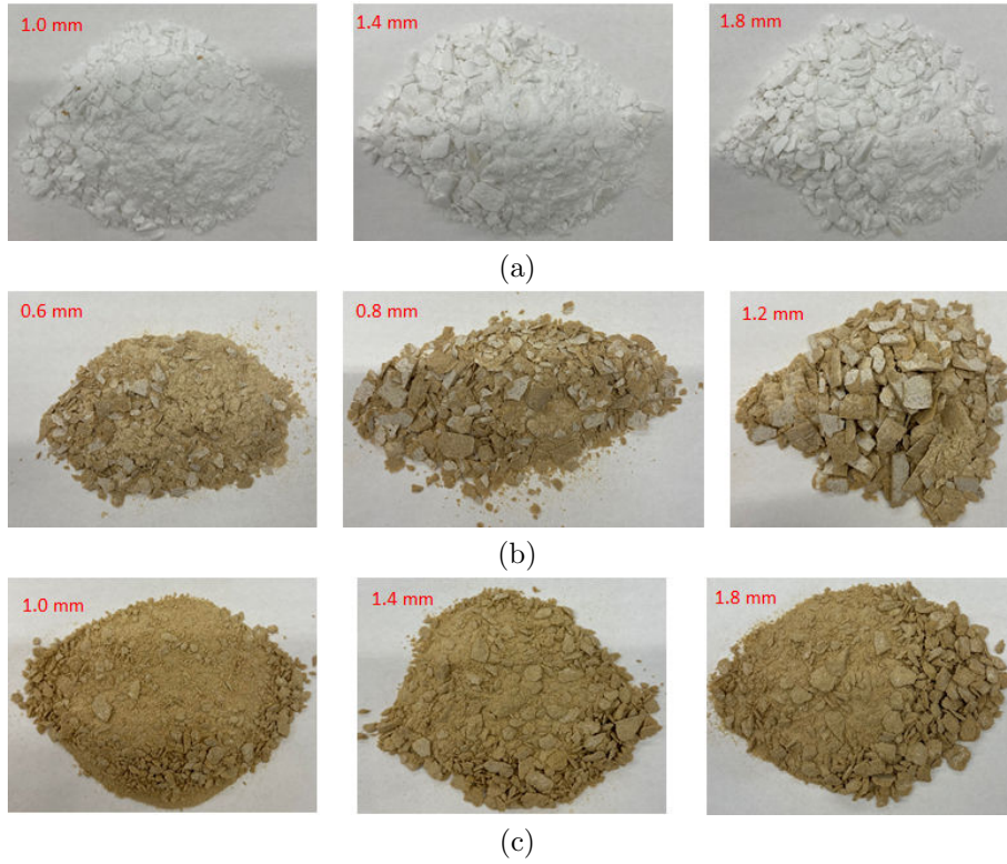
Figure 8: Collection of the rock cuttings for: (a) Alabama Marble, (b) Bonne Terre Dolomite and (c) Dunnville Sandstone, each at three different depths of cut.
