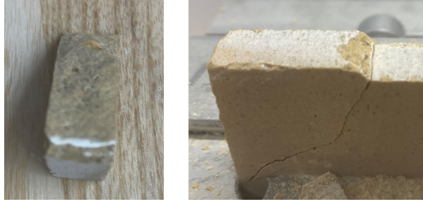
Figure 17: Powdery appearance at the trailing edge of a rock chip as evidence for the formation of the crushed zone at the cutter tip.
