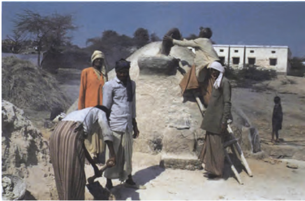
FIG. 9. Prepared batch is introduced into the furnace through rectangular filling-hole. (Photo: from Sode and Kock 2001, 166, fig. 10)
