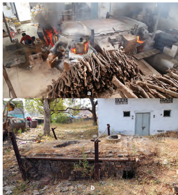
FIG. 14. (a) Glassworking furnace and (b) abandoned furnace at Kapadwanj. (Photo: Alok Kanungo)
