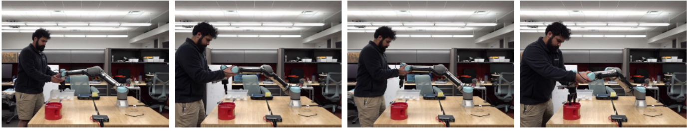
Fig. 14. Operator demonstrating a pick-and-place task to a UR5e robot without obstacles.
