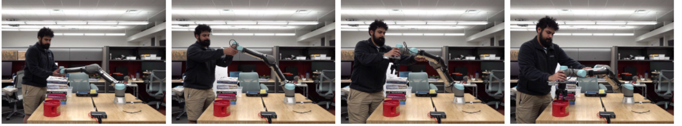
Fig. 15. Operator demonstrating a pick-and-place task to a UR5e robot with an obstacle.
