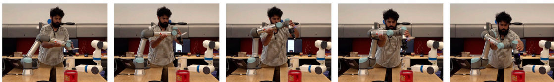
FIGURE 13 | A human teacher demonstrating the pick-and-place task to a UR5e robot.
