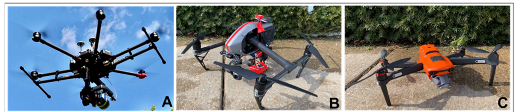
Figure 2. UAS sensor combinations used in the study: (A) DJI Matrice 600 Pro with Headwall Nano-Hyperspec VNIR and Velodyne Puck lite LiDAR sensors, (B) DJI Inspire II with MicaSense Rededge multispectral sensor, and (C) Autel Evo II with Sony 1" CMOS 20 RGB sensor.
