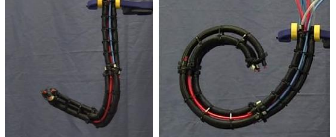
Fig. 1. A illustration of a 3-section continuum arm achieving different spatial shapes.
