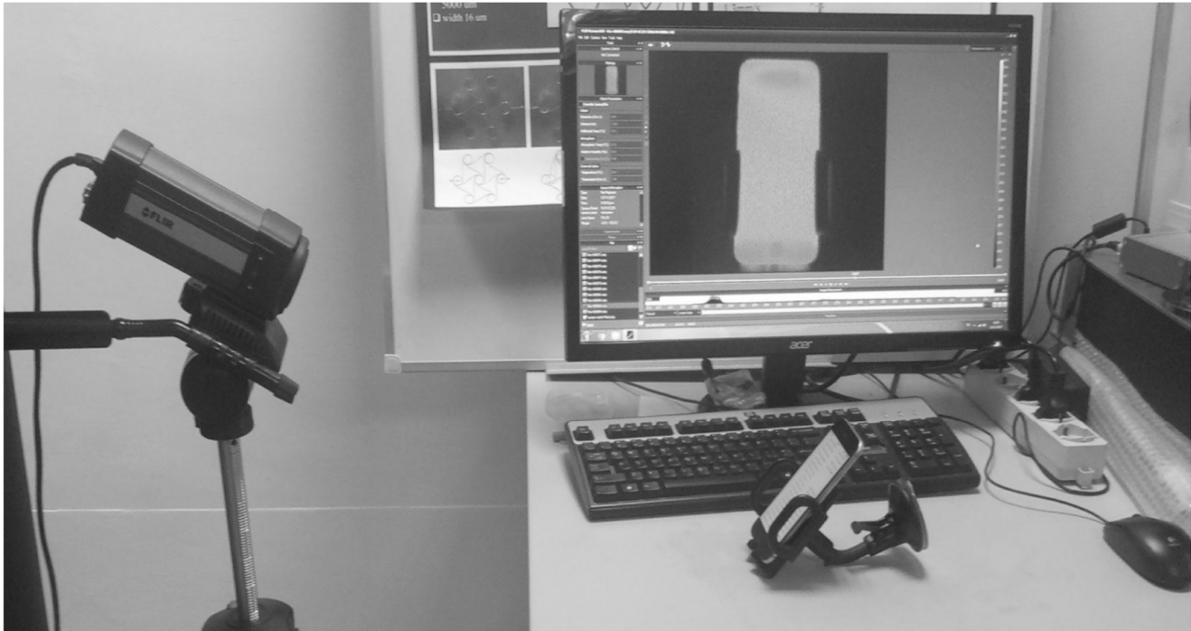
Fig. 2 The experimental setup with the thermal camera, smartphone, and data processing workstation. On the monitor screen the thermal field is visible.
