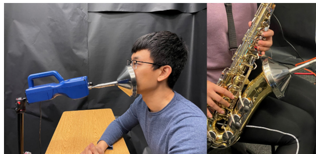
FIGURE 4 Source aerosol measurements with funnels for singing (left) and instrument (right)
