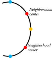
Fig. 2. The procedure of the closest point projection performed on yield patches. In the case where the admissible stress lands in the overlapped domain of two patches, the mean of the admissible stress will be used as the stress update. Note that the consistency requirement enforced by Eq. (10) should ensure that the difference between these two stress measures remains negligible.
