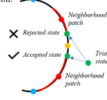
Fig. 2. The procedure of the closest point projection performed on yield patches. In the case where the admissible stress lands in the overlapped domain of two patches, the mean of the admissible stress will be used as the stress update. Note that the consistency requirement enforced by Eq. (10) should ensure that the difference between these two stress measures remains negligible.
