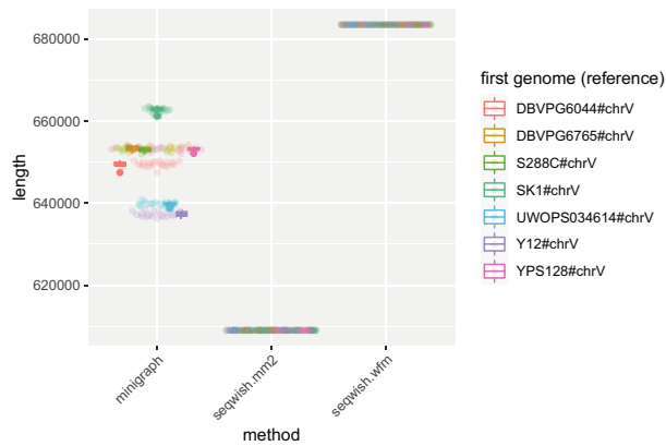
Fig. 3. Base-pair lengths of graphs built from 100 permutations of yeast chrV. Each point corresponds to the length of a graph built from a specific permutation and the given method. We color each point by the first genome in the order (the ‘reference’ in minigraph ). A boxplot per first genome group provides the mean and the first and third quartile intervals for each reference grouping
