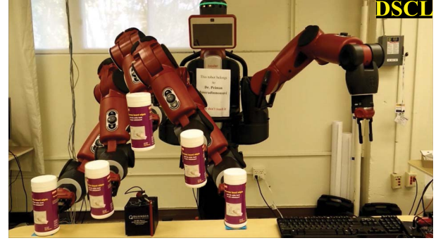
Fig. 12. Baxter performing a pick-and-place task while subjected to an input delay of 0.9 s (0-s initial delay estimate).
