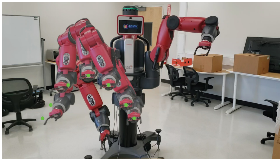
Fig. 3 Baxter tracking a desired trajectory under the prescribed-time control scheme, correcting for a large initial tracking error of 20 degrees in each joint and attenuating a sinusoidal torque disturbance of D(t) = 0.1\sin(5t) . The circles represent the reference trajectory to be tracked, and are spaced at approximately 1 s intervals.
