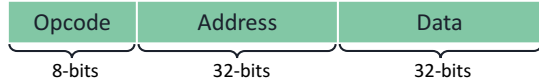
Figure 4: Hardware Fuzzing Instruction. A bus-centric harness (test-bench) reads binary Hardware Fuzzing Instructions from a fuzzer-generated test file, decodes them, and performs TL-UL bus transactions to drive the DUT (Fig.13). Our Hardware Fuzzing Instructions comprise a grammar (Tbl. 1) that aid syntax-blind coverage-guided greybox fuzzers in generating valid bus-transactions to fuzz hardware.
