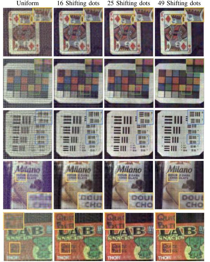
Fig. 7: Experimental results on five test scenes with different numbers of shifting dots patterns. The reconstruction results using multiple coded illumination patterns outperform the standard lensless camera with uniform illumination. The quality of reconstruction gradually increases as the number of illumination patterns increases.
