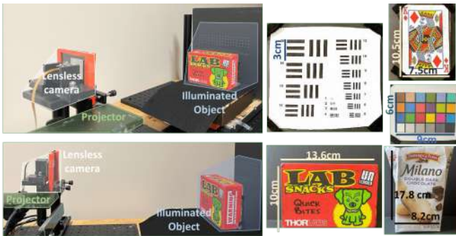
Fig. 6: The experiment setup and five test scenes (annotated and scaled to proportional size). The projector is placed right next to the lensless camera. The target scenes/objects are 40cm away from the camera.
