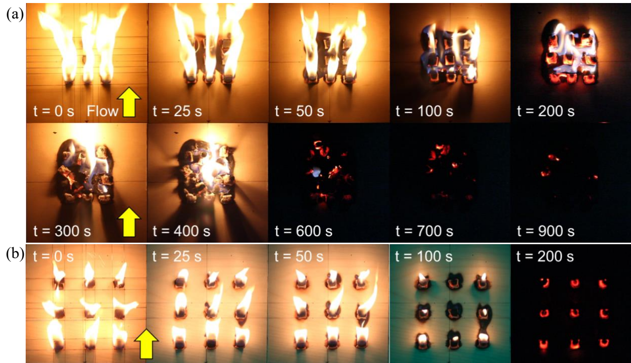
Figure 2. Sequential images of the experiments since the firebrands drop (defined as t = 0 s) under u = 0.5 m/s (a) s = 10 mm and (b) s = 30 mm. (wind direction is from bottom to up)
