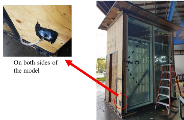
Figure 4. Vented Cavity DSF (Courtesy of WOW Research Team)
