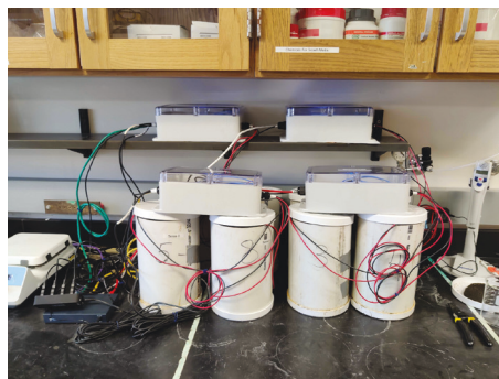
FIGURE 2. (a) Diagram of a microbial fuel cell with carbon felt electrodes. Initially there is no potential, but as a microbial biofilm forms, power output rises. (b) A photograph of cells in the laboratory. After 60 days, the biofilm is able to provide a consistent output of 15-25 \mu\text{W} .
