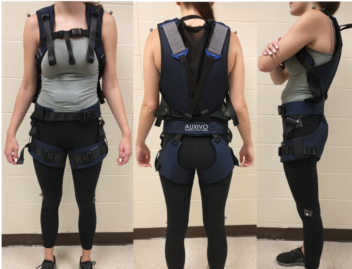
Fig. 1. A participant wearing the Auxivo LiftSuit (Auxivo AG, Switzerland): front, back and side views. The participant is also wearing the sensors used in the study (e.g., wireless electromyography sensors under shirt, optical tracking markers on shoulders, hips and knees).
