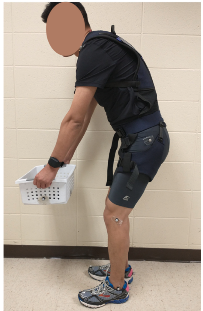
Fig. 2. A participant lifting a box from the floor while wearing the exosuit and sensors. Optical tracking markers are visible on the body and box. Electromyography sensors are not visible from this angle.
