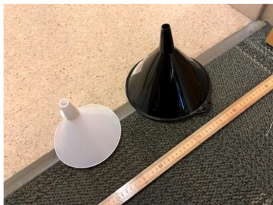
FIG. 8. (Color online) (a) A screenshot from the BIAS software showing the measurement of two input impedance curves for simplified trumpets using two different funnels. The vertical axis is in acoustic megohms; the scale is linear. The horizontal axis is frequency. The two funnels were similarly shaped although different in size. The two impedance curves are nearly identical. (b) A photo of the two differently sized but similarly shaped funnels.
