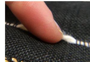
floats of a length specific to each material will spring back to shape after being pressed. We call this the sweet spot.
