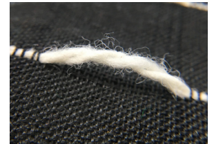
floats of a length specific to each material will spring back to shape after being pressed. We call this the sweet spot.
