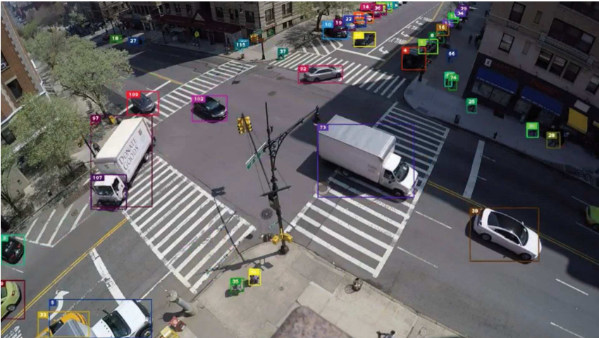
FIGURE 5. Pedestrian and vehicle detection on 120th Street and Amsterdam Avenue, fourth floor view.
