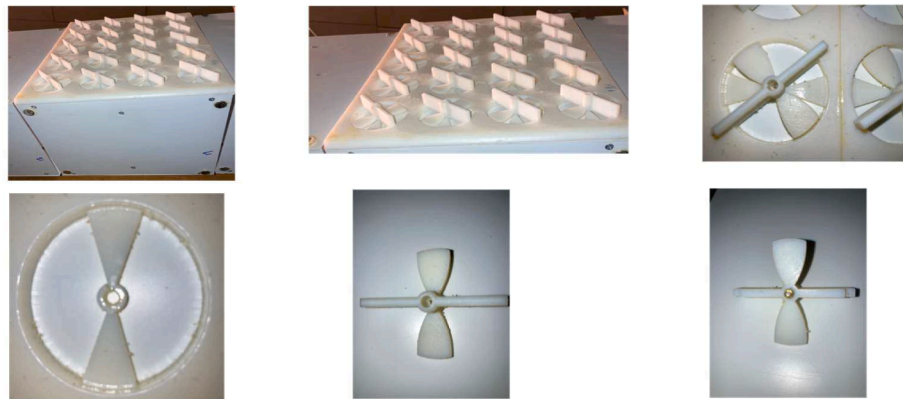
(c) (clockwise from top left): a typical panel mounted on one wall of the model, the perpendicular wall is exposed to show magnetic buttons used for mount; closeup view of the panel; closeup view of one assembled unit of the panel; stationary fan unit; front view of the rotating fan unit with fins; rear view of the rotating fan unit with fins
