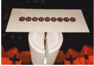
Fig. 19. A photograph of the fabricated 9-element, dual-mode linear array antenna under test in an anechoic chamber.
